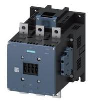
power contactor, AC-3e/AC-3 400 A, 200 kW / 400 V AC (50-60 Hz) / DC Uc: 220-240 V 3-pole, auxiliary contacts 2 NO + 2 NC drive: conventional main circuit: busbar control and auxiliary circuit: screw terminal
